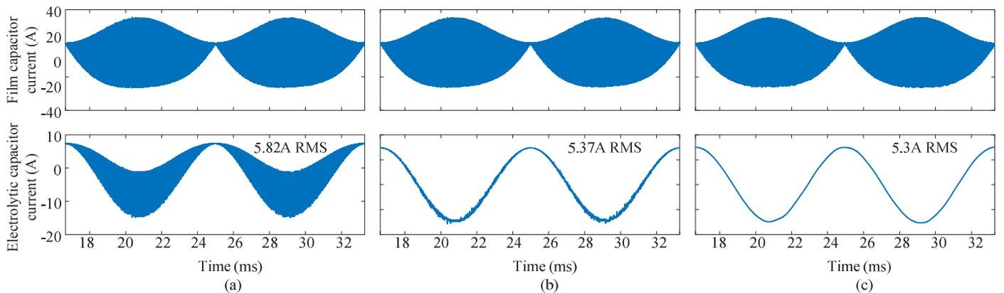
Fig. 6 Current sharing performance: (a)  $L_E = 10\text{nH}$ ; (b)  $L_E = 3.3\mu\text{H}$ ; (c)  $L_E = 1.25\text{mH}$ .
