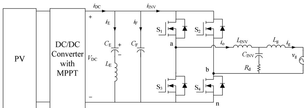
Fig. 1 Grid-tied single-phase PV inverter with a hybrid capacitor bank.
