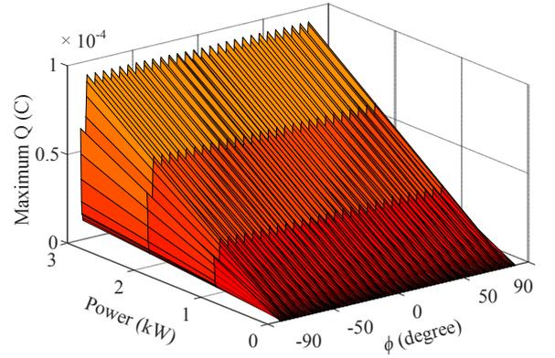
Fig. 3 Maximum Q for calculating the film capacitor.
