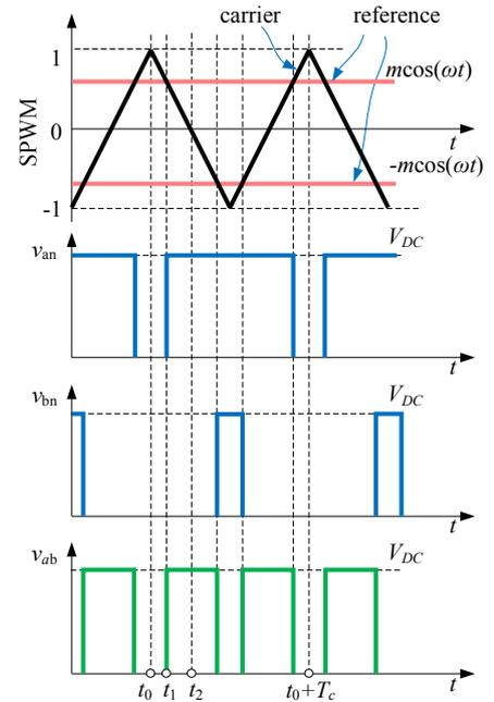
Fig. 2 Unipolar SPWM modulation illustration.
