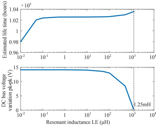
Fig. 5 Estimated lifetime of the electrolytic capacitor and DC-bus voltage variation with different resonant inductance  $L_E$ .
