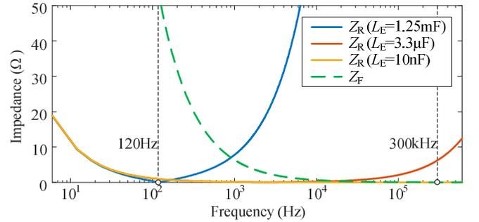
Fig. 4 Impedance of the resonant filter and film capacitor.
